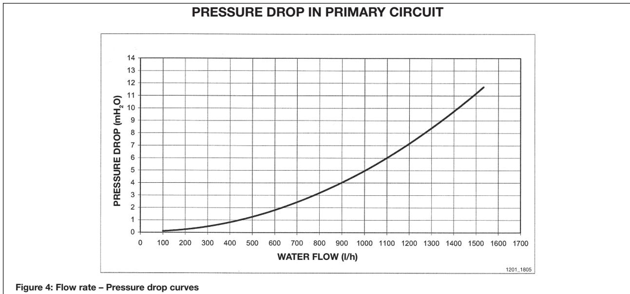
Figure 4: Flow rate - Pressure drop curves
