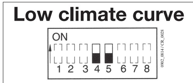
This selection allows central heating temperature to be adjusted by turning the heating water adjustment potentiometer (TCH) on the electronic board. The temperature range is 25 - 40 °C.
