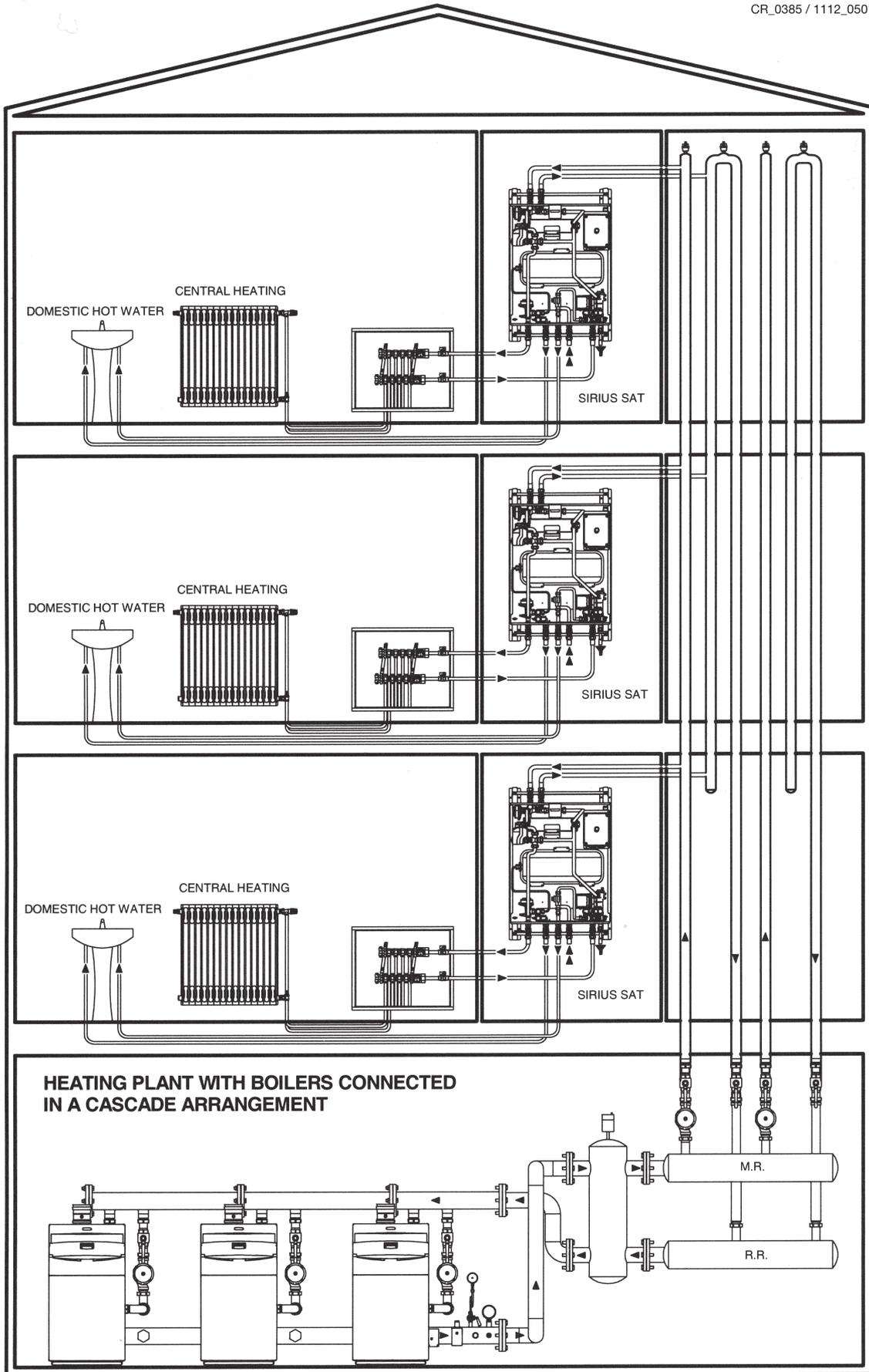
Figure 1A: Diagram of plant: local domestic hot water production
