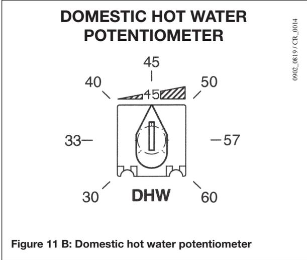
Figure 11 B: Domestic hot water potentiometer
