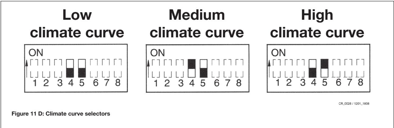
Figure 11 D: Climate curve selectors
