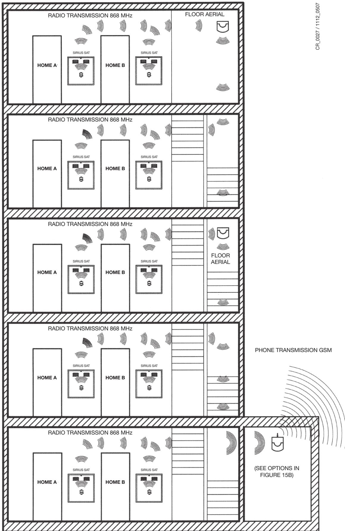
Figure 13 A: Automatic measurement system via radio
