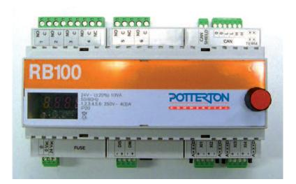
The RB100 acts as an interface between the DDC, and on-site BMS systems where it will accept a heat request from a BMS as a VFC or a 0-10Vdc input to automatically provide a compensated flow temperature.
